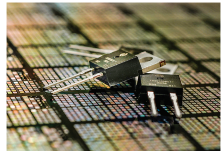
iDEAL Semiconductor's diodes rest on a wafer containing about 30,000 small silicon die.
